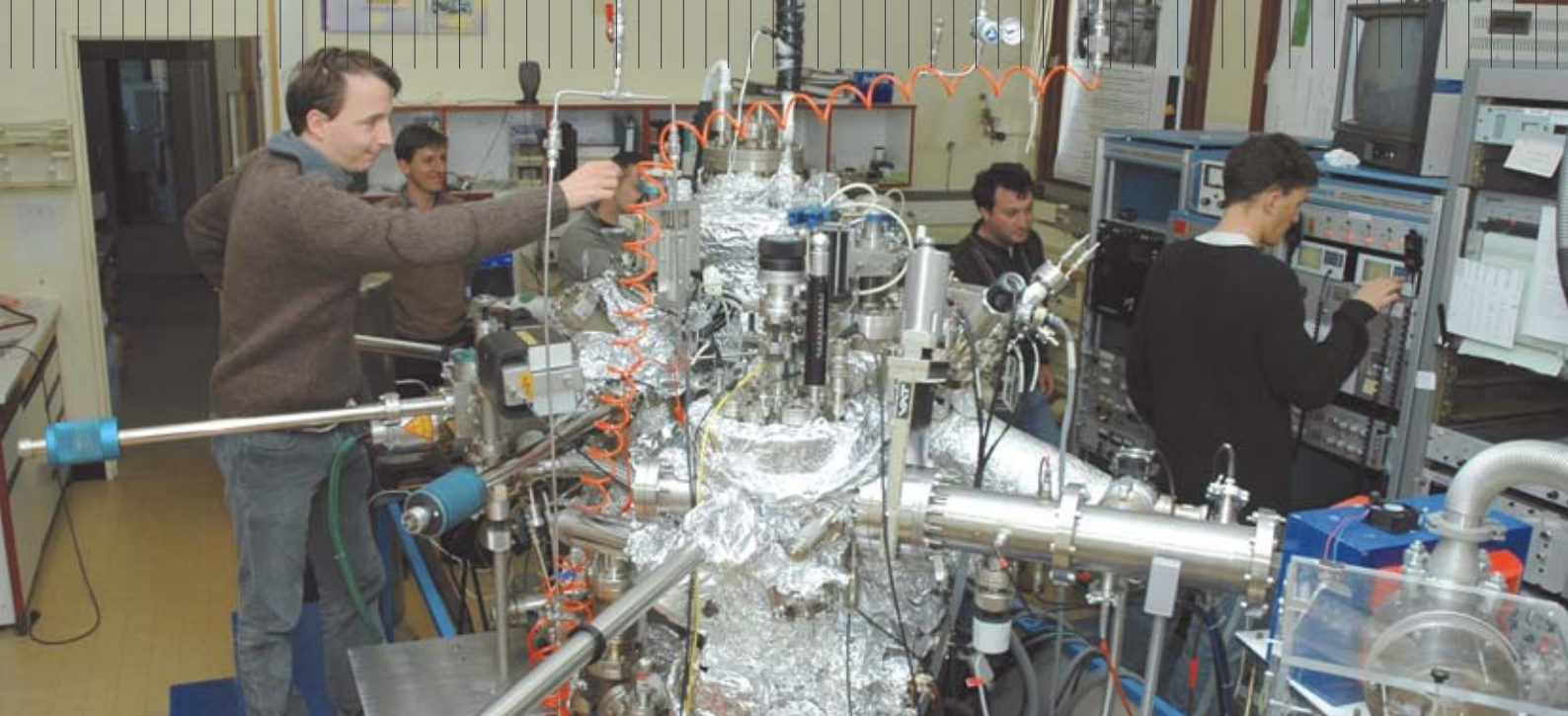
Epitaxy of magnetic layers with perpendicular anisotropy carried out at the Laboratory of Nanostructures and Magnetism, CEA Grenoble (Isère).
